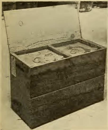
Standard two-can shipping case with strong partition in middle between the cans. Each 5-gal. can holds 60 lbs. of honey.
